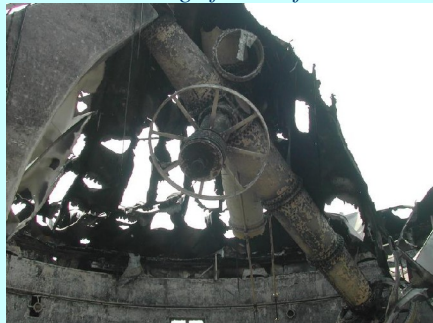
Remains of the Yale-Columbia Refractor after the 2003 fire. Photographs by Matthew Colless, RSAA, Australian National University
