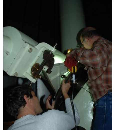
Basil Rowe (left) & Kirk Schrotel lubricate the 16-inch Clark telescope
